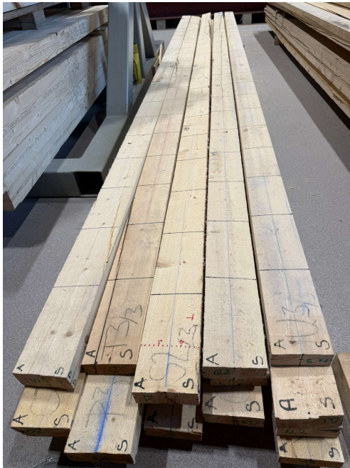
Photo 3.2-1 Reclaimed timber beams used in the study prior to testing
