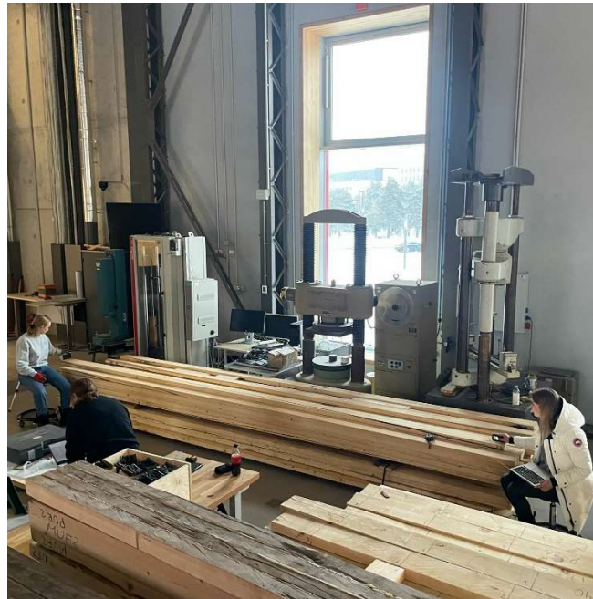
Photo 3.2-2 Measurement of specimen geometry and documentation of visual defects
